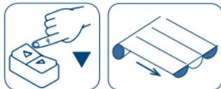
Pressing one of the two buttons and releasing, the motor drives to the desired direction until it reaches the limits.
