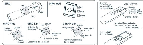
To prevent accidental changes to the programming of the motor during the daily use of the remote control, the possibility of programming is disabled automatically 8 hours after sending the last sequence (A+B or B+C).
