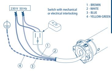
WIRE PROGRAMMING - only for motors up to 25 Nm -
