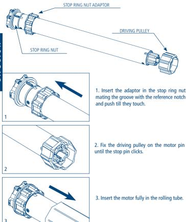
**NB:** If you use tubes with a round form, the driving pulley must be fixed to the tube, and the installation is to be paid by the person who installs the system. For other tube sections the fitting is optional, but strongly recommended.
