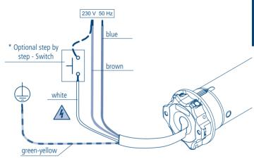
\* Installing this button is optional. The connection can be done differently using the brown wire or the blue wire. The button affords the possibility to command the motor in stepping mode (up, stop, down, stop, up, stop, down, stop..)
