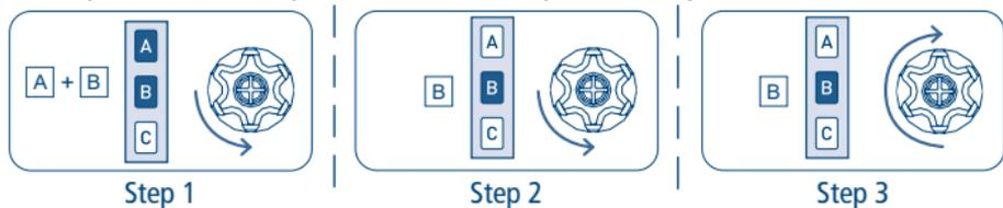
As we can see from the example, when the sequence ends positively, the motor returns to its starting position in one long rotation. In fact, two short rotations in the same direction correspond to one long rotation in the opposite direction. The motor returns to the starting position even when the sequence is not completed; in this case by performing one or two short rotations. Example of a wrong sequence:
