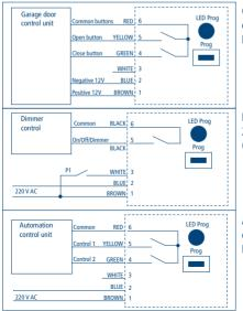
Garage door control unit controlled by BT 2 outputs Domotic RX
