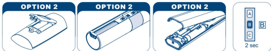
Remove one battery and wait minimum 5 seconds or press any button.
