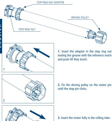
**NB:** If you use tubes with a round form, the driving pulley must be fixed to the tube, and the installation is to be paid by the person who installs the system. For other tube sections the fitting is optional, but strongly recommended.
