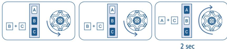
At the end of the sequence, wait until the rolling shutter is completely lowered. From this moment onwards the motor moves in "Dead Man" mode. This enables the regulation of the positions to be adjusted precisely.
