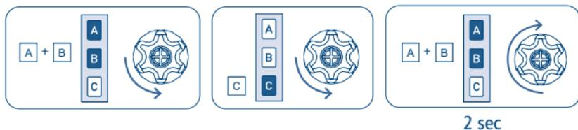
The total deletion of the limit switches automatically resets the short slat tilting adjustment impulse.
