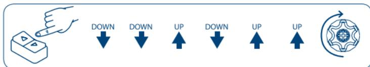
The total deletion of the limit switch automatically resets the short slat tilting adjustment impulse.
