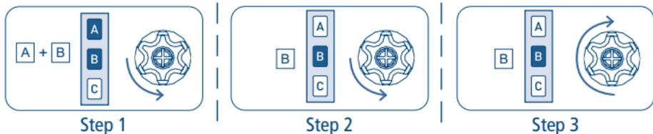
As we can see from the example, when the sequence ends positively, the motor returns to its starting position in one long rotation. In fact, two short rotations in the same direction correspond to one long rotation in the opposite direction. The motor returns to the starting position even when the sequence is not completed; in this case by performing one or two short rotations. Example of a wrong sequence:
