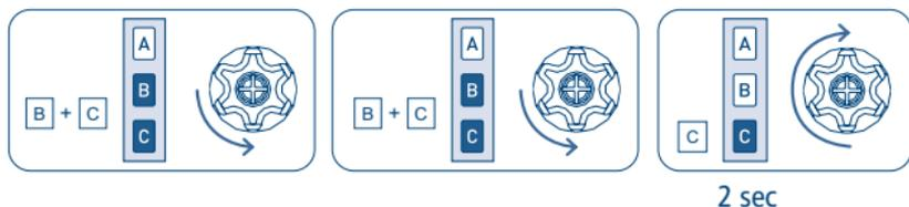
At the end of the sequence, wait until the rolling shutter is completely lowered. From this moment onwards the motor moves in "Dead Man" mode. This enables the opening positions to be adjusted precisely.
