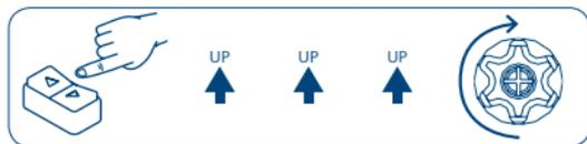
As we can see from the example, when the sequence ends positively, the motor carries out one long rotation.
