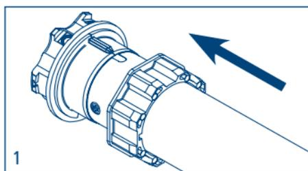
1. Insert the adaptor in the stop ring nut mating the groove with the reference notch and push till they touch.
