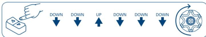
After deletion of the limit switches the radio function automatically resets.
