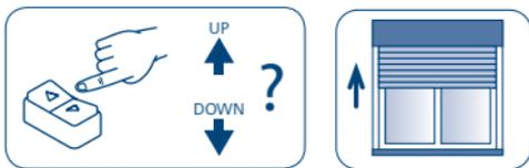
Follow the command sequence given in order to save the opening position. At the end of the sequence, the motor carries out a short "down" movement which confirms that the settings have been saved and then it brings back the shutter to the opening position.
