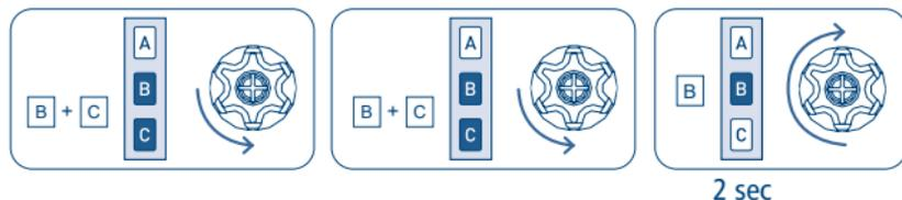
At the end of the sequence, wait until the rolling shutter is completely lowered. From this moment onwards the motor moves in "Dead Man" mode. This enables the regulation of the positions to be adjusted precisely.
