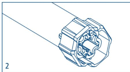
2. Fix the driving pulley on the motor pin until the stop pin clicks.
