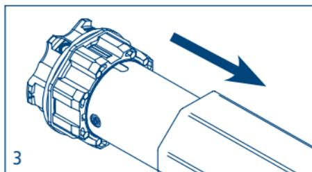
3. Insert the motor fully in the rolling tube.
