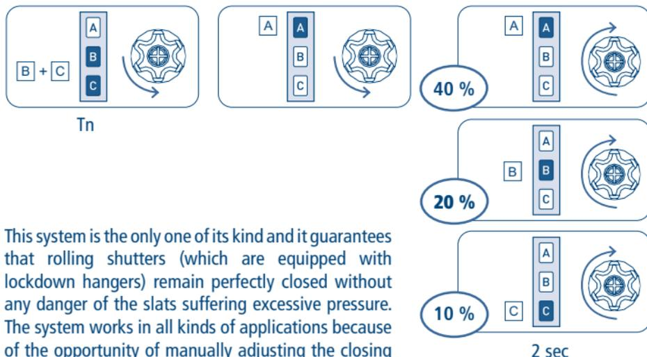
This system is the only one of its kind and it guarantees that rolling shutters (which are equipped with lockdown hangers) remain perfectly closed without any danger of the slats suffering excessive pressure. The system works in all kinds of applications because of the opportunity of manually adjusting the closing force.
