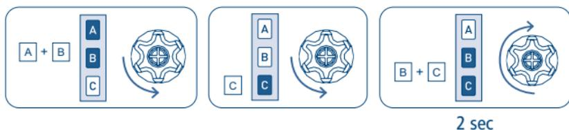
in this way fewer impulses will be needed to adjust the opening of the slats from their minimum to their maximum.
