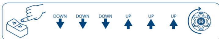
After the sequence the motor will go into "Dead Man" mode so as to enable the exact adjustment of the middle position desired. To memorise the position chosen, confirm with this sequence:
