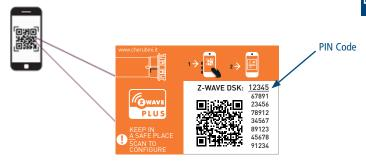
The PIN code of the Z-Wave Device Specific Key (DSK) is required when adding the DIMIO ZRX to a Z-Wave network with a controller supporting Security 2 Autenticated (S2). The unique DSK code is printed on the product label. The first five digits of the key are highlighted and underlined to help the user identify the PIN code portion of the DSK text.
