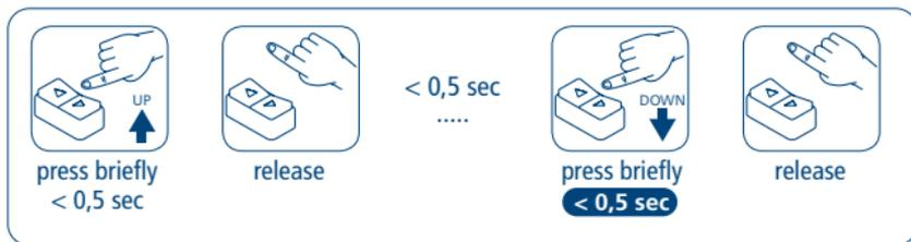
Using the switch as described on this page it's possible to set the motor trough the white wire (WIRE PROGRAMMING).
